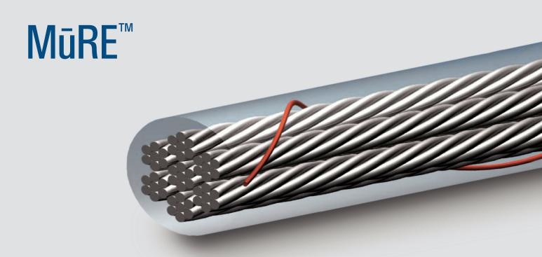
MūRE™ is a permanent reference electrode for *reinforced* concrete structures to detect corrosion in early stage. It is made of a series of linear-Ni-made-electrodes, working as pseudo-reference electrodes to measure the local potential of steel reinforcements.
